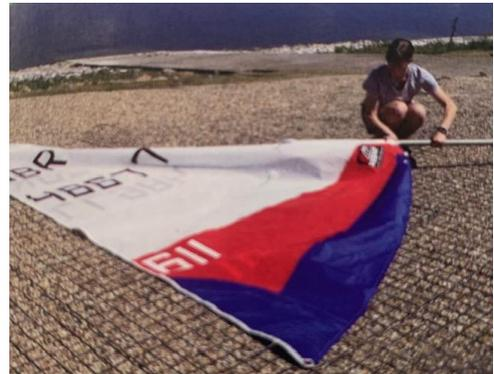
3. Push the mast into the sail sleeve until the whole sail is sleeved and mast-head has appeared at the top.
